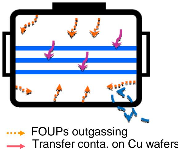
HCl transfer kinetic to Cu-coated wafer after FOUPs intentional contamination and purge step [\*]
