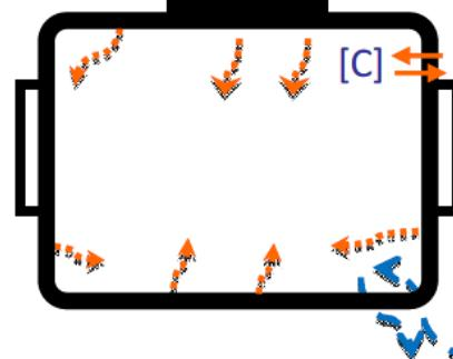
Contamination transfer FOUP → Air → Wafer
