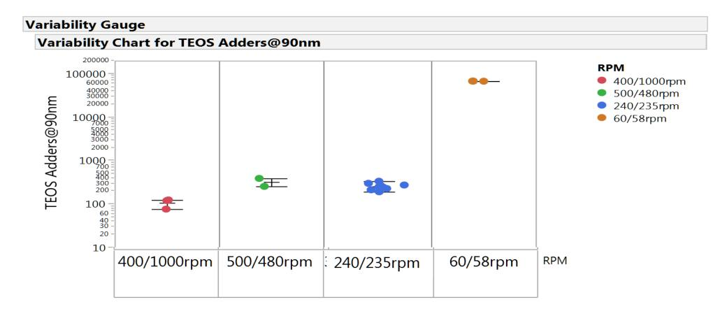
High rotation speed with mismatched wafer / pad speeds shows improved performance
