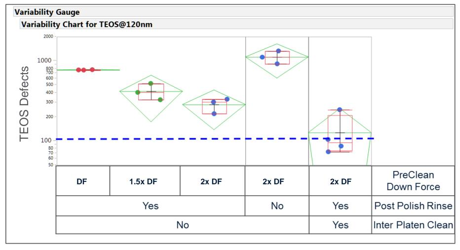
Both Polish and Clean processes must be optimized to achieve best defect performance: Post Polish Wafer Rinse and IPC significantly improved defect results High shear rate Pre-Clean process ensures high particle removal efficiency
