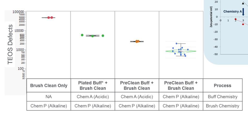
Pre-Clean buff with alkaline chemistry shows best defect performance, as expected based on Zeta-potential Diagram
