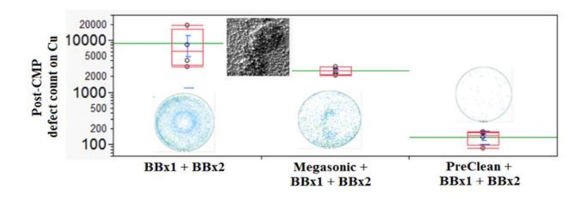
Pre-Clean removes particles and organic residue from Cu polished with a challenging slurry
