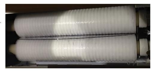
Two consecutive brush boxes provide high particle removal efficiency and precise brush pressure control
