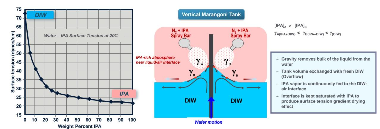
Vertical Marangoni Dryer provides defect-free drying of hydrophilic, hydrophobic and mixed surfaces
