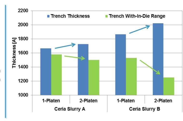
Lower Topography and WID Range by Controlling Pad Temp and By-product Defectivity challenge: No platen available to perform Buff
