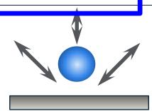
Diffusion of particles to surface due to overall attraction force and electrostatic force
