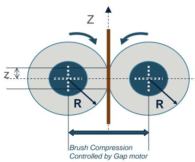
$$F_{shear} = \mu F_{normal} = \mu PA$$
