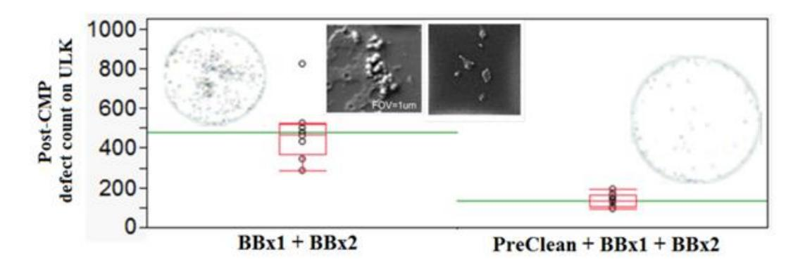
Pre-Clean effectively removes residues from hydrophobic ULK surface
