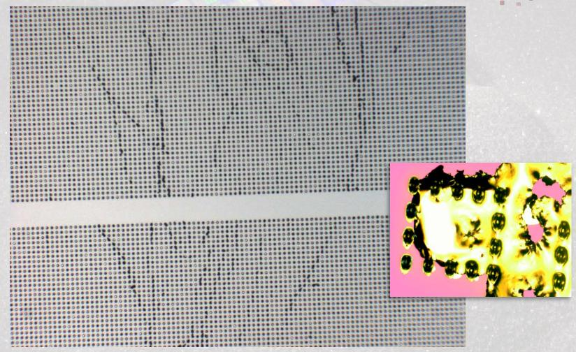
Damage due to rolling of metal as it was removed and rubbed the tops off the bumps
