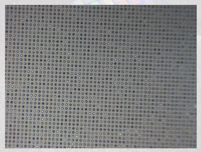
Good cleaning but slight rubbing during removal creates shine on the tops of the bumps
