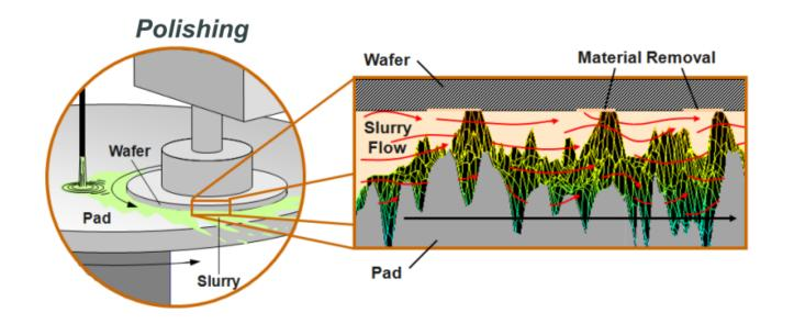
Pad's pores and grooves allow the slurry transport while the contact with the wafer is determined by its pores and asperities. In this study we
