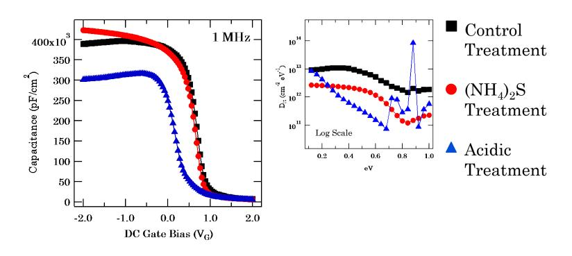
Flatband shift possibly due to thickness of dielectric layer.
