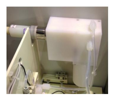
Internal check valve design to prevent down stream water backflow causing contamination on membrane and DI water supply
