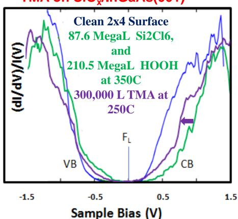
Left: STS on n-type InGaAs: clean n-type InGaAs (2x4), 87.6 MegaL Si2Cl6 + 210.5 MegaL HOOH at 350C (ave of 7 curves), 300,000 L TMA at 250C (ave of 11 Curves)
