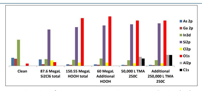
XPS Spectra collected at 30° glancing angle. Corrected XPS peak areas for clean (2x4), and following 87.6 MegaLangmuir  $Si_2Cl_6$  at 350°C, 150.55 MegaLangmuir HOOH at 350°C, 60 MegaLangmuir additional HOOH at 350°C, 50,000 L TMA at 250°C, and additional 250,000 L TMA at 250°C.  $Si_2Cl_6$  pulses at 2.5x10^-2 Torr . HOOH pulses at 1x10^-2Torr . TMA pulses at 5x10^-3 Torr .
