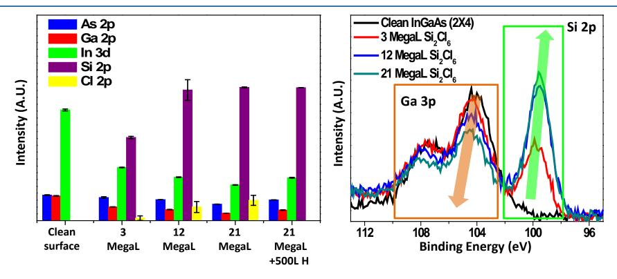
Left: XPS Spectra collected at 30° glancing angle. Corrected XPS peak areas for clean (2x4), and following 3, 12, and 21 MegaLangmuir total Si<sub>2</sub>Cl<sub>6</sub> doses at 350°C.(Si<sub>2</sub>Cl<sub>6</sub> dosed at 10 second pulses of 0.025 Torr).
