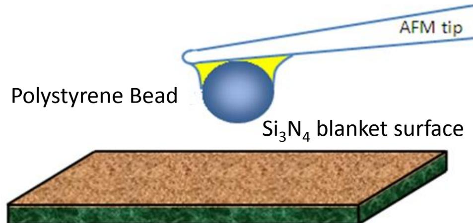
A technique using AFM (atomic force microscopy) was developed to measure the adhesion forces between colloidal silica particles (50 – 80 nm) and wafer surfaces in the cleaning solution. Additionally, by attaching a polystyrene bead (~5 $\mu$ m) to the AFM cantilever and measuring the force-distance curve to Si<sub>3</sub>N<sub>4</sub>, Cu and W wafers the adhesion force between polystyrene and the wafer substrate was obtained.
