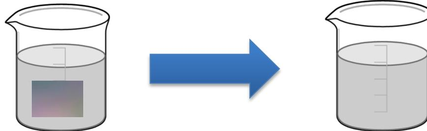
Immerse the tungsten coupon for 10 minutes in the cleaning solution
